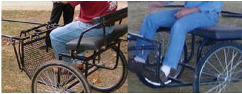
Notice the difference of entering the carts and the center of gravity or height of the seat.
